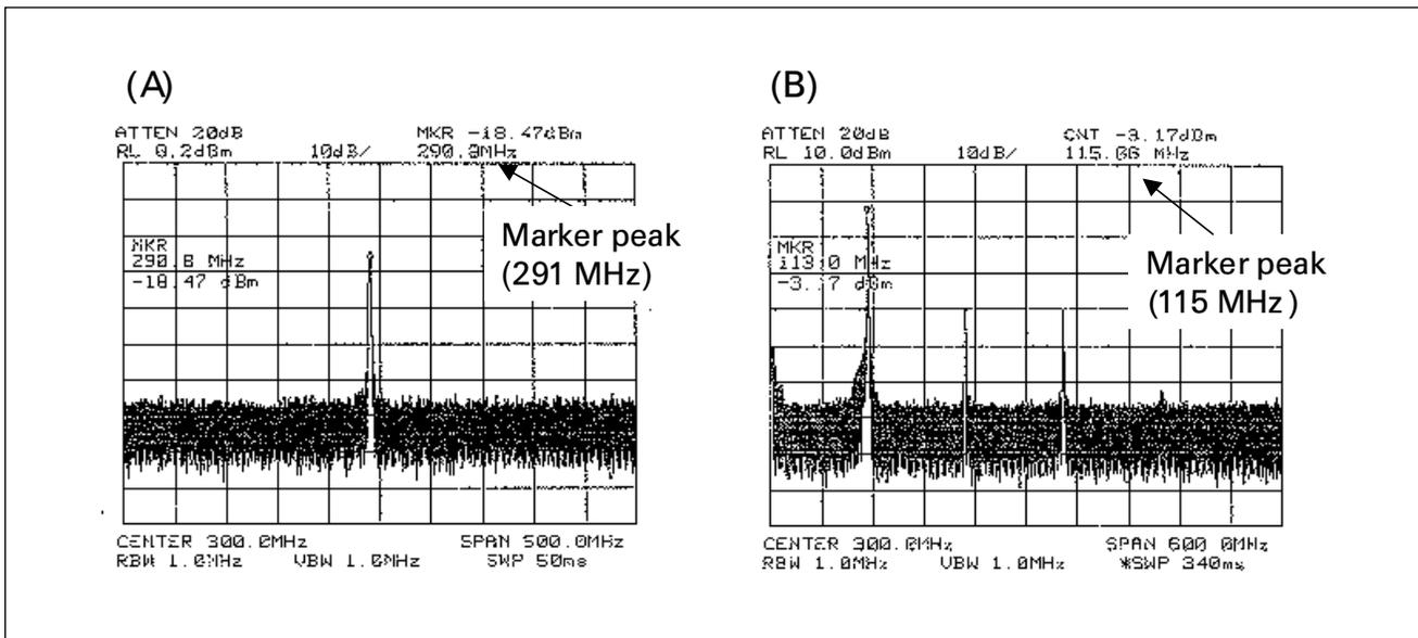
Figure 3. Example of ring oscillator evaluation results at 291 MHz (A) and 115 MHz (B)
