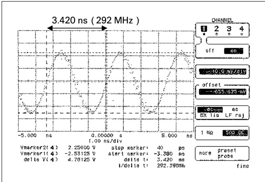
**Figure 1. Waveform of a ring oscillator through the switching matrix of the Agilent 4072A Parametric Tester**
