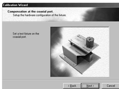
Figure 11. Calibration wizard (fixture connection after calibration)
