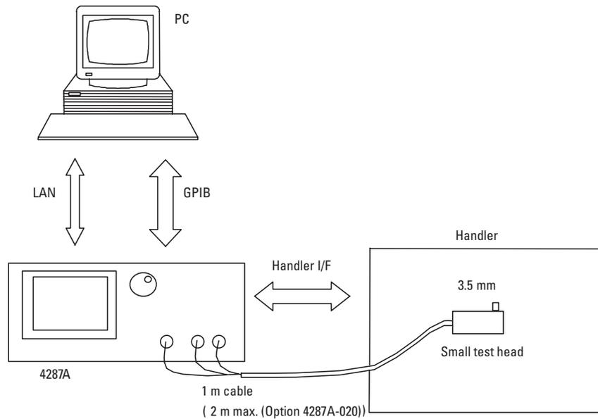
Figure 7. Handler system example with the 4287A
