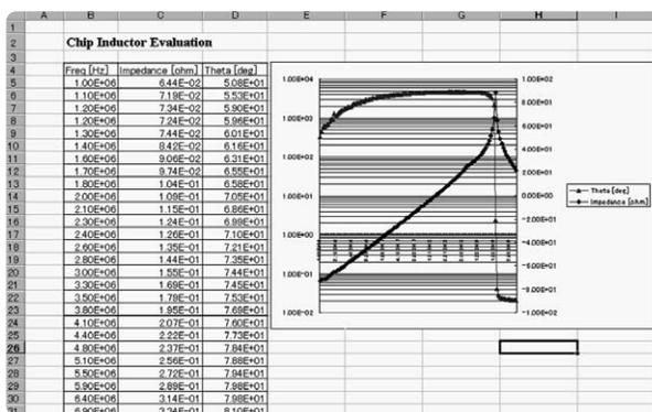
Figure 13. Frequency characteristics plot using spreadsheet software
