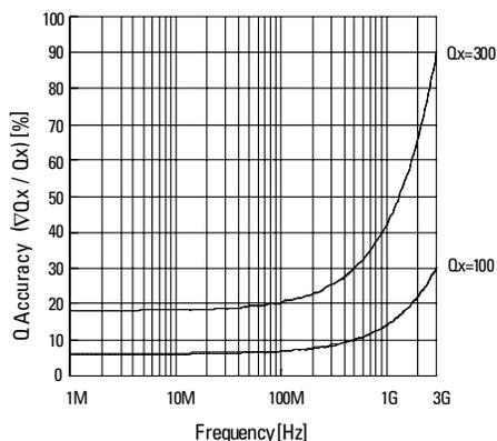
Figure 10. Q accuracy @ 7-mm port (typical)
