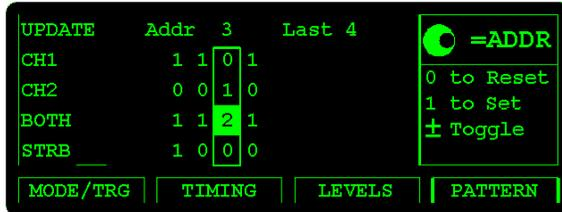
**STEP 2:** Set up the bit pattern as shown above in the PATTERN menu. Start with setting the LAST bit to 4.
