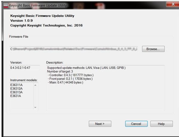
5. Select the I/O interface (LAN, USB, or GPIB) that connects the instrument to your PC.
