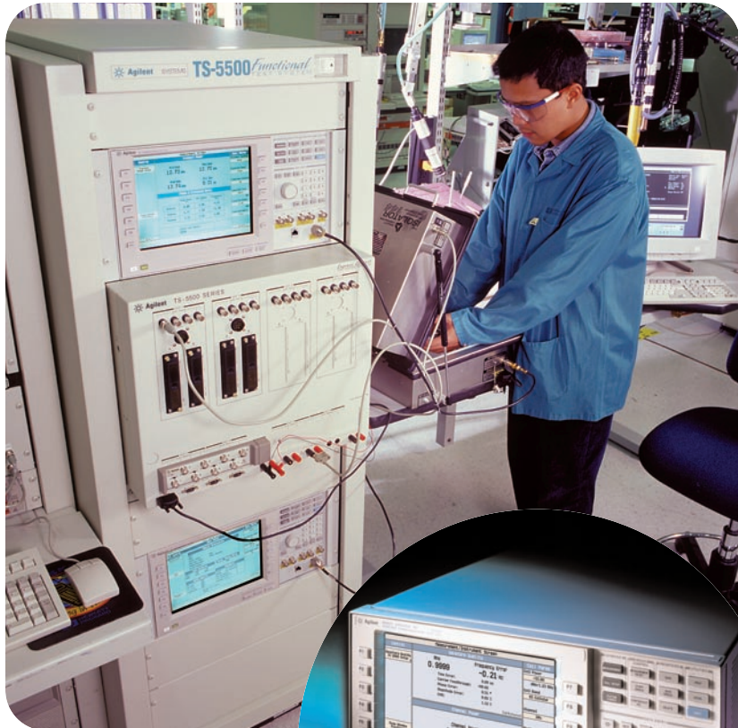
Agilent E1985A GSM, GPRS, W-CDMA and AMPS_136 mobile test application (fast switching) and 8960 Series 10 wireless communications test set
