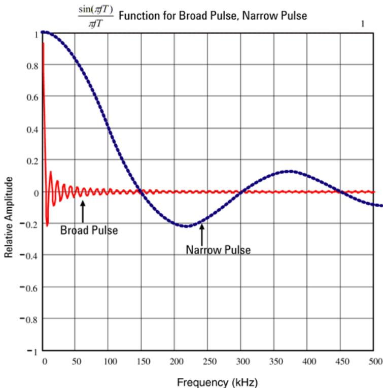
Figure 2. Fourier integral of two different pulses
