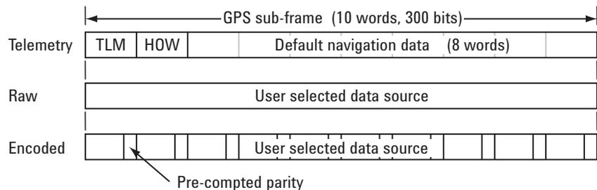
Figure 1. Sub-frame structure for the data modes
