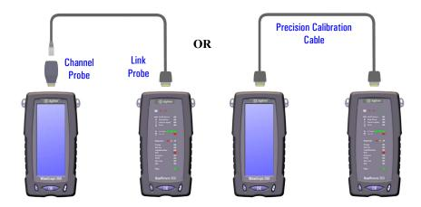
If you are testing link configurations to Category 6 / Class E or higher, Agilent Technologies recommends that you use the precision calibration cable, as this produces the most accurate calibration.
