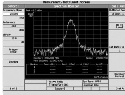
**Use the general-purpose spectrum monitor to view signals while on a call.**
