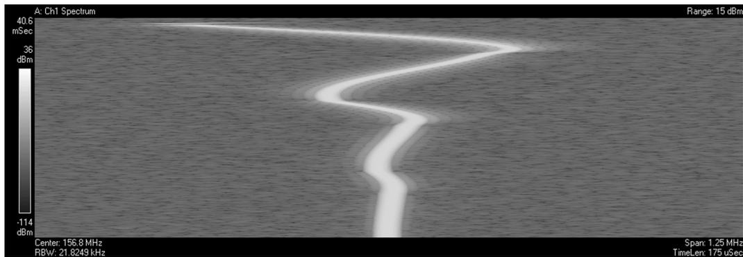
Figure 9. Spectrogram display of a VCO turn-on transient
