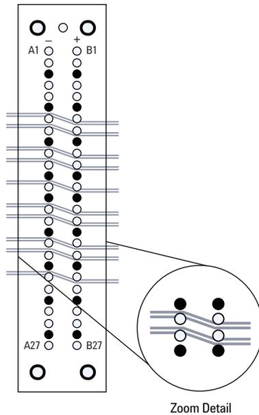
**Figure 4. Recommended RapidIO board routing for probe connection**
