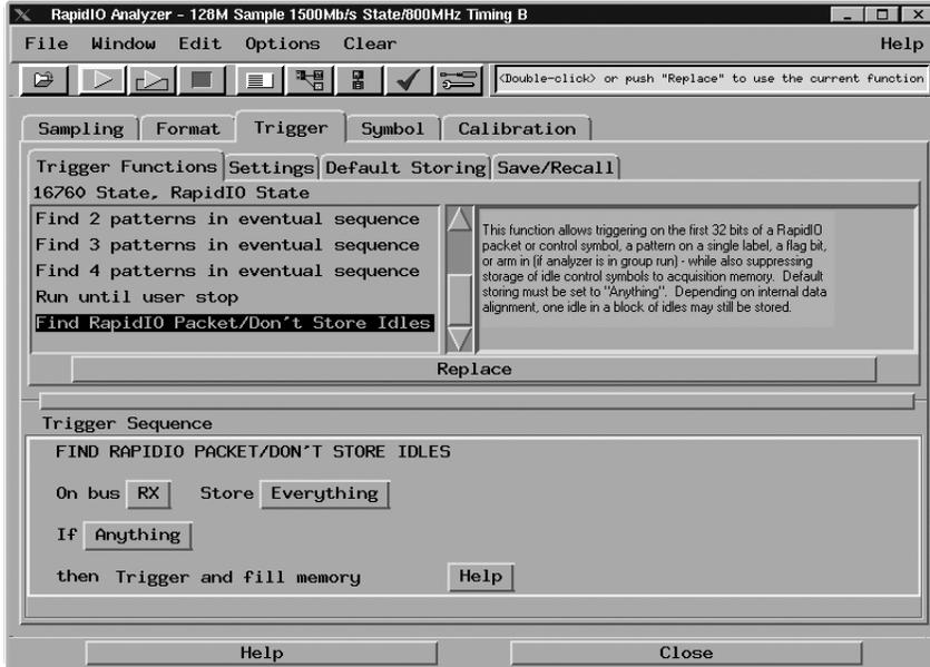
Figure 18. Trigger menu in logic analyzer setup window
