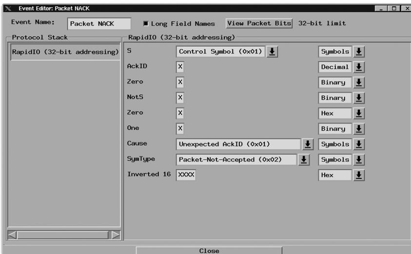
Figure 21. A Control Symbol trigger for a Packet Not Accepted because of an Unexpected AckID
