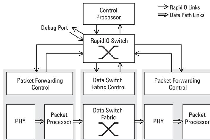
**Figure 1. Example IP router design with RapidIO interconnects**
