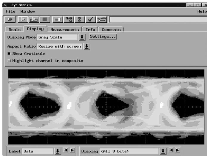
Figure 11. Eye diagrams collected on all signals simultaneously
