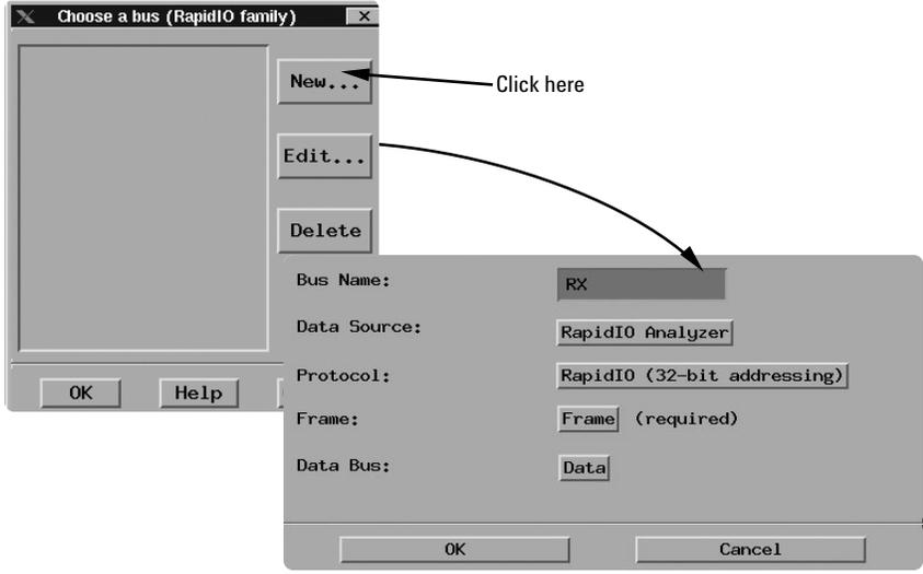
Figure 16. Bus selector setup
