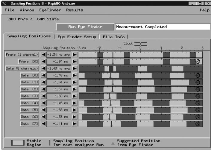
**Figure 13. "Run Eye Finder" computes the data stable regions relative to the clock edges and automatically configures the sampling positions for each bus channel**
