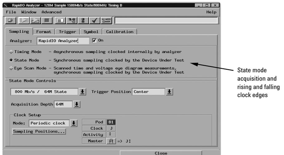
Figure 12. State mode configuration showing sampling on rising and falling clock edges
