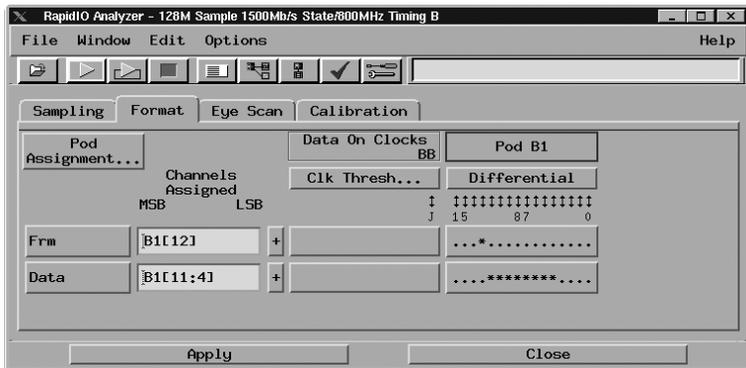
**Figure 9. Format menu connecting bus signals to logic analysis pods and channels**
