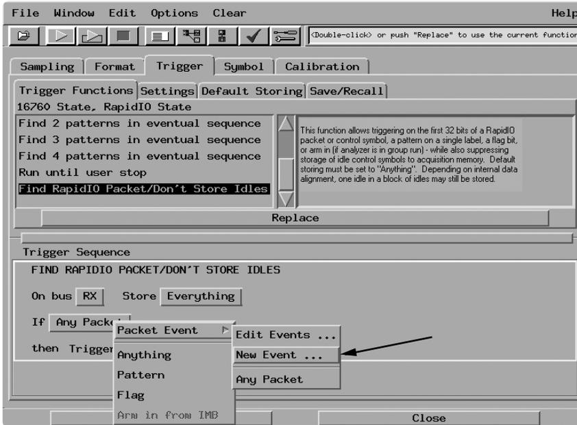
Figure 19. "New Event" button for setting triggers on specific packet or control symbol protocols
