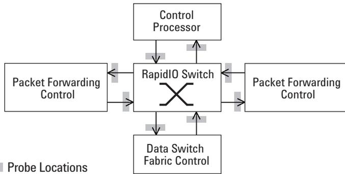
**Figure 3. Probe connection locations**
