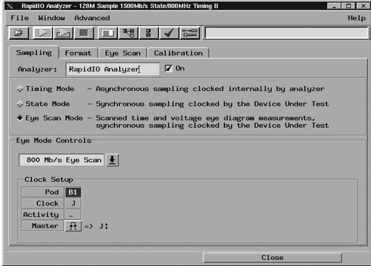
**Figure 8. Sampling configuration of 16760A logic analyzer using both rising and falling clock edges**
