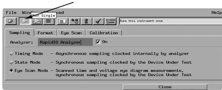
Figure 10. Setup for eye scan mode with arrow pointing to start button
