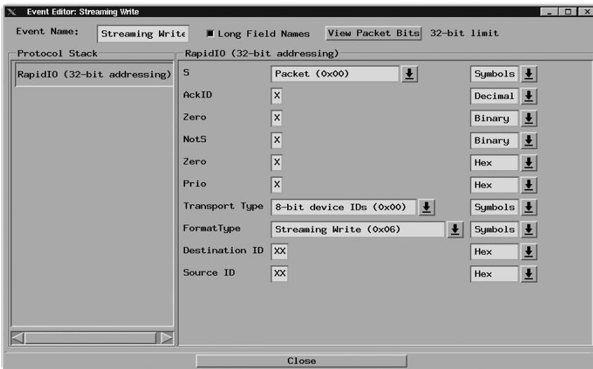
Figure 20. Trigger setting for a streaming write packet
