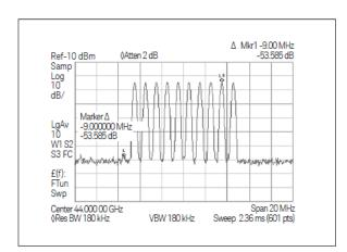
20 GHz image rejection (measured)
