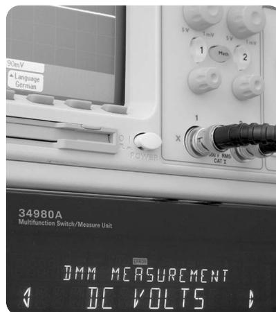
Figure 2. Agilent 34980A multifunction switch/measure unit
