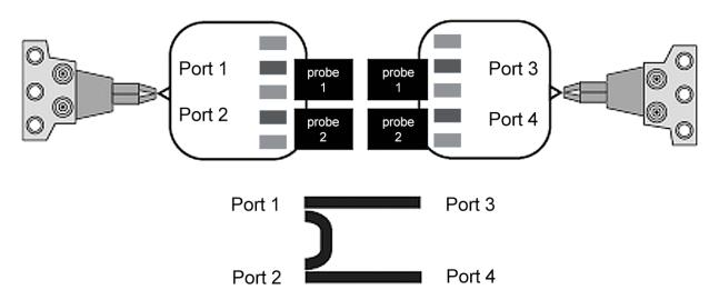
**Figure 6a.** Assigning test ports as either probe 1 or probe 2 offers the PNA-L the most efficient way of executing minimum thru. This example allows the PNA-L to maximize the number of straight thrus and minimize the number of non-straight ones.
