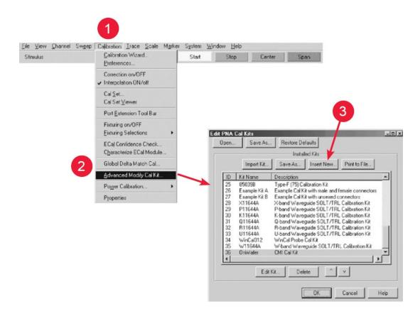
Figure 5. Creating a new calibration kit for probing.
