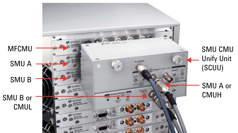
Figure 3. Accurate IV and CV measurement setup using SMU, MFCMU and SCUU.
