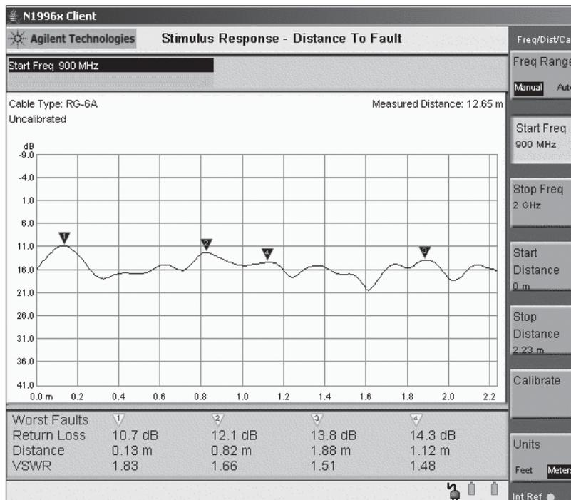
Figure 1. Distance-to-fault measurement
