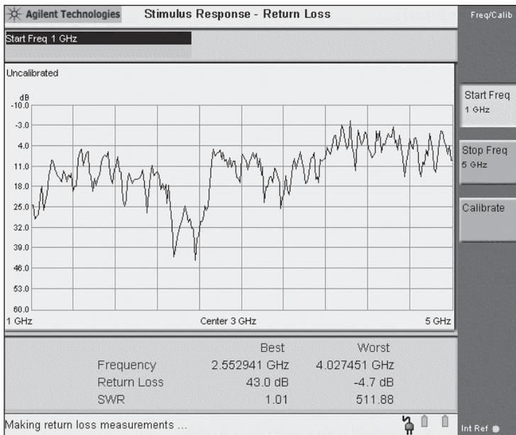
Figure 3. Return loss measurement
