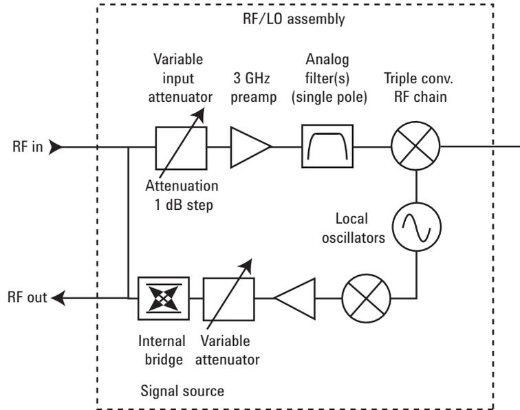
Figure 4. Highly integrated RF/LO board with internal signal source and bridge
