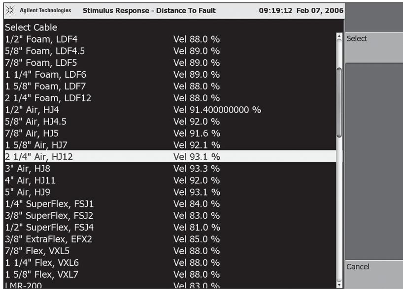
Figure 6. Built-in cable type selection for measurement setup
