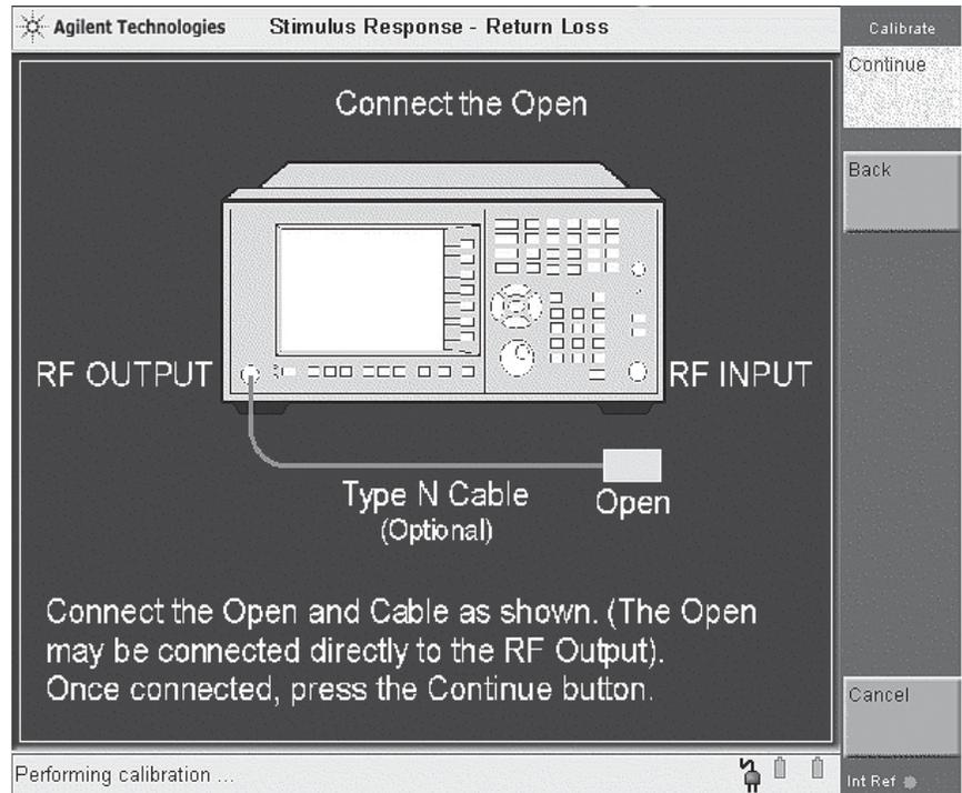
Figure 5. Screen shot of calibration help diagram
