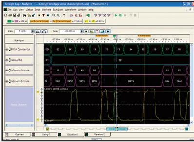
Instantly validate the logical and timing relationships between the analog and digital portions of your design by viewing analog and digital waveforms integrated into a single logic analyzer display.
