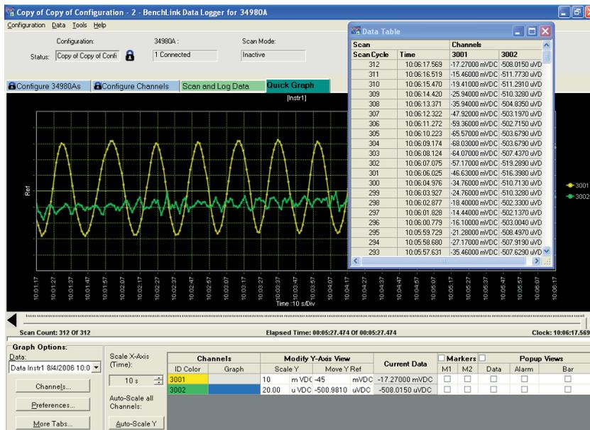
The Keysight Technologies BenchLink Data Logger software provides a convenient way to collect and analyze your data. This software is a Windows-based application that uses a familiar spreadsheet environment to define measurement data to be collected. The tab-based format makes it easy to set up and initiate scans. Simply identify the measurements you want to acquire, initiate the process, and see the data displayed real-time.
