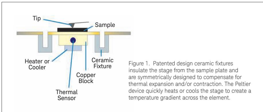
Figure 1. Patented design ceramic fixtures insulate the stage from the sample plate and are symmetrically designed to compensate for thermal expansion and/or contraction. The Peltier device quickly heats or cools the stage to create a temperature gradient across the element.
