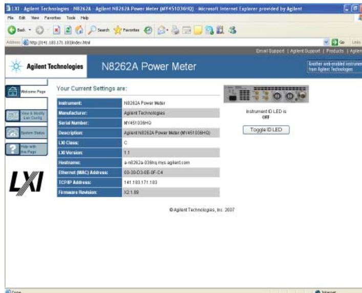
Figure 6. Instrument Webpage browser that provides instrument setting at a glance and enable remote access/control
