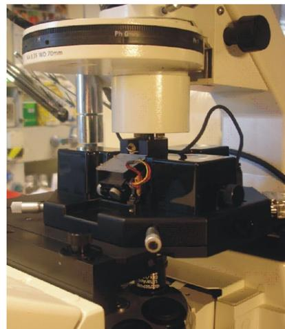
Figure 2. Keysight 5500 ILM AFM/SPM with a Zeiss Axiovert 200 inverted light microscope. The 5500 ILM AFM/SPM is also compatible with other inverted light microscope makes and models.
