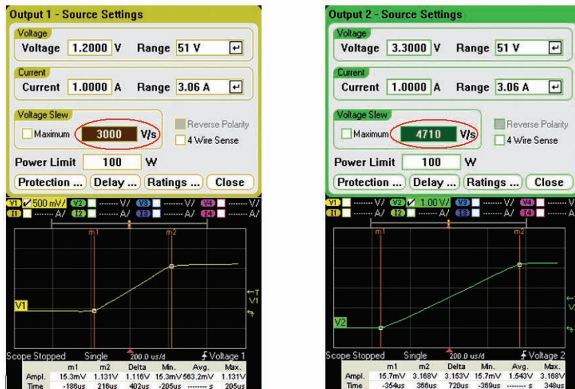
Figure 4. Core voltage and I/O voltage slew rate settings
