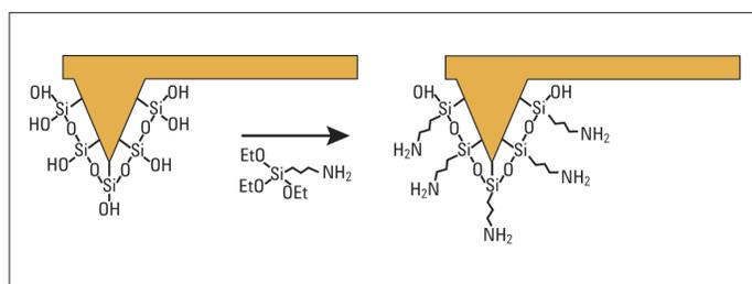
Figure 4. Amination of MAC levers with aminopropyltriethoxysilane (APTES).
