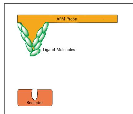
Figure 1. Direct immobilization of ligands to the tip of an AFM probe. This type of immobilization can often lead to a high density of molecules on the probe, but these ligands are generally not able to diffuse within a defined volume of space nor are they able to reorient and bind with the receptors in an optimal manner.
