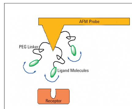
Figure 2. Ligand immobilization with PEG linkers. The PEG linker confines the ligands within a defined volume of space and they have enough flexibility and freedom to diffuse, then reorient and bind with their complimentary receptors in an optimal manner.
