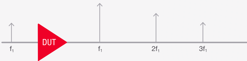
A single tone stimulus signal produces harmonics
