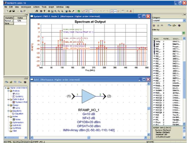
▲ Fig. 4 Improved system modeling with 20<sup>th</sup> order intermodulation terms and hybrid S-n nonlinear models.
