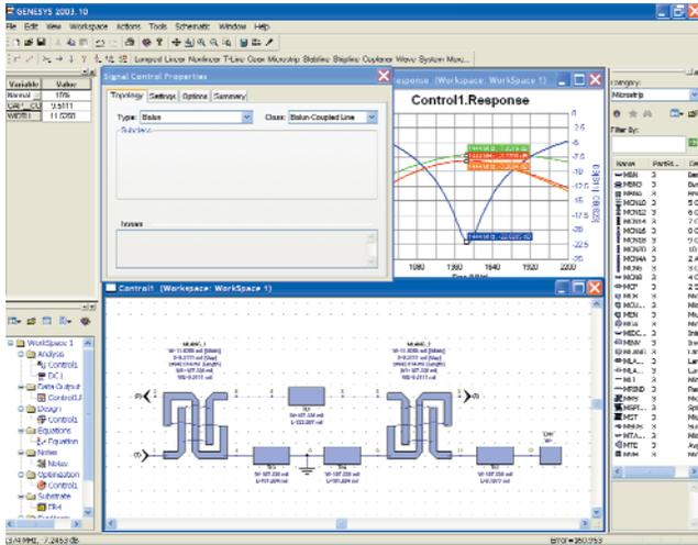
▲ Fig. 2 SIGNAL CONTROL synthesis to speed and simplify the design of couplers and splitters.
