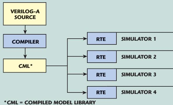
▲ Fig. 1 Flow from a single Verilog-A source to multiple simulators.
