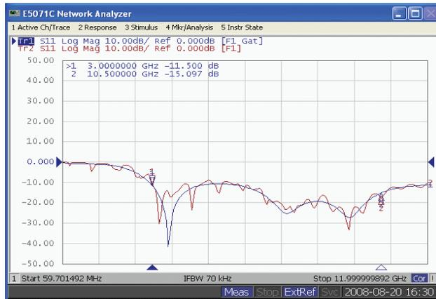
Figure 4. Frequency domain with/without gating
