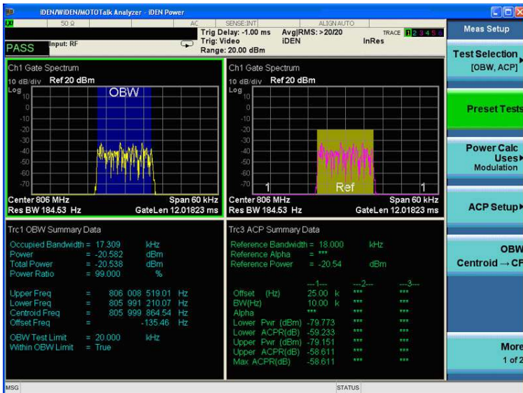
Figure 4. N6149A iDEN power and frequency measurements
