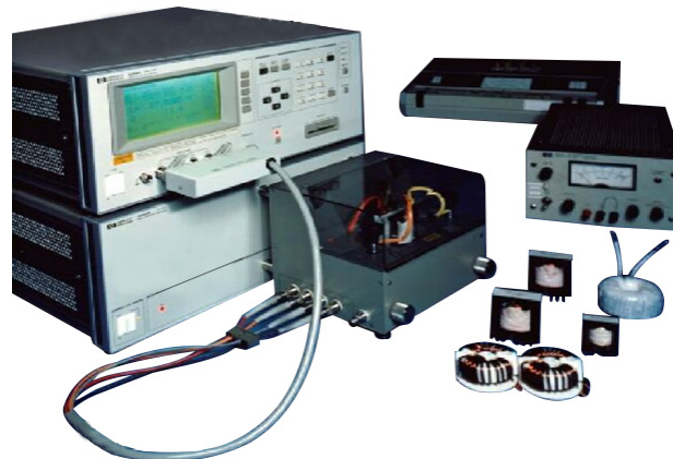
Measurement using 42841A bias current source
