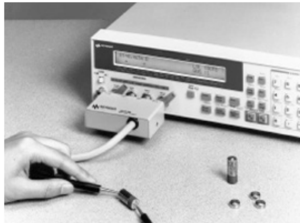
Internal resistance tests for batteries
