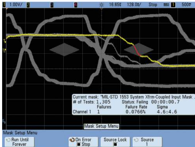
Figure 8: A “stop-on-error” mask test uncovers a bit shift error.
