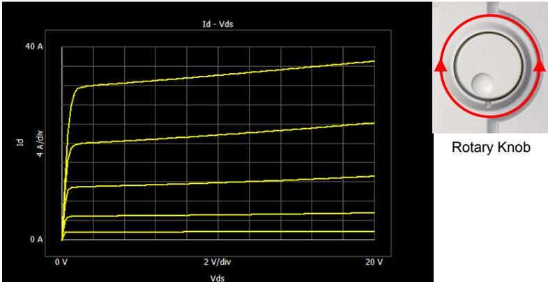
Figure 7. Example  $I_d$ - $V_{ds}$  characteristics of a packaged power MOSFET measured in Tracer Test mode.  $V_{ds}$  is swept from 0 V to 40 V, and  $V_{gs}$  is stepped from 2.0 V to 2.8 V in 0.2 V steps.
