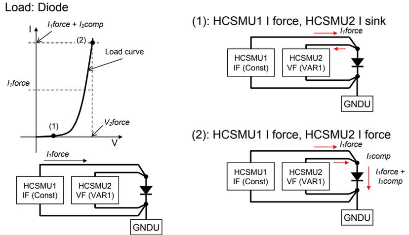
Figure 3. VF mode operation example using two HCSMUs in parallel
