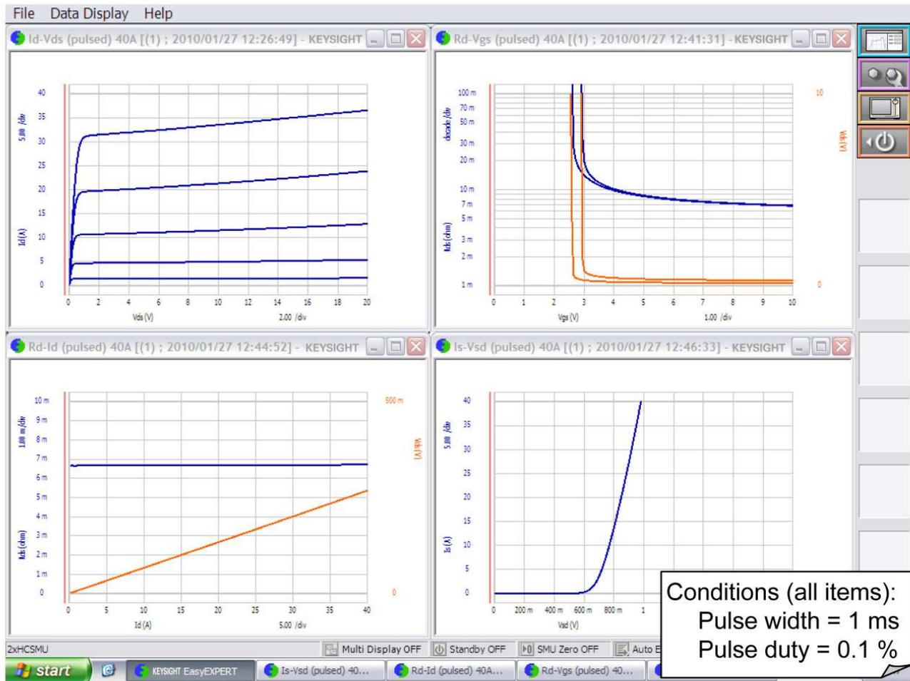
Figure 8. Sample  $R_{ds(on)}$  measurements of a packaged power MOSFET ( $R_{ds(on)} \approx 8 \text{ m}\Omega$ ). Plots show the  $I_d$ - $V_{ds}$ ,  $R_{ds}$ - $V_{gs}$ ,  $R_{ds}$ - $I_d$ , and  $I_s$ - $V_{sd}$  characteristics.
