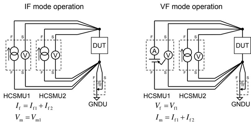
Figure 2. Block diagram of current force (IF) and voltage force (VF) modes using two HCSMUs in parallel.
