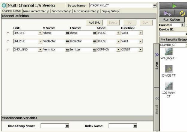
(a) Test parameter setup window of Classic Test
