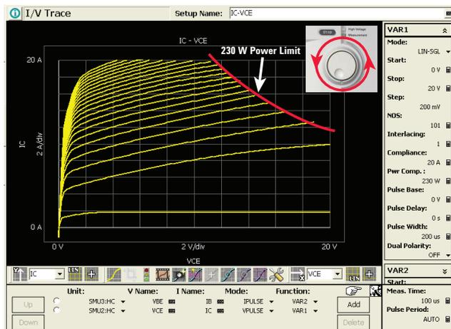
Figure 3.  $I_c$   $V_{ce}$  Tracer Test example.
