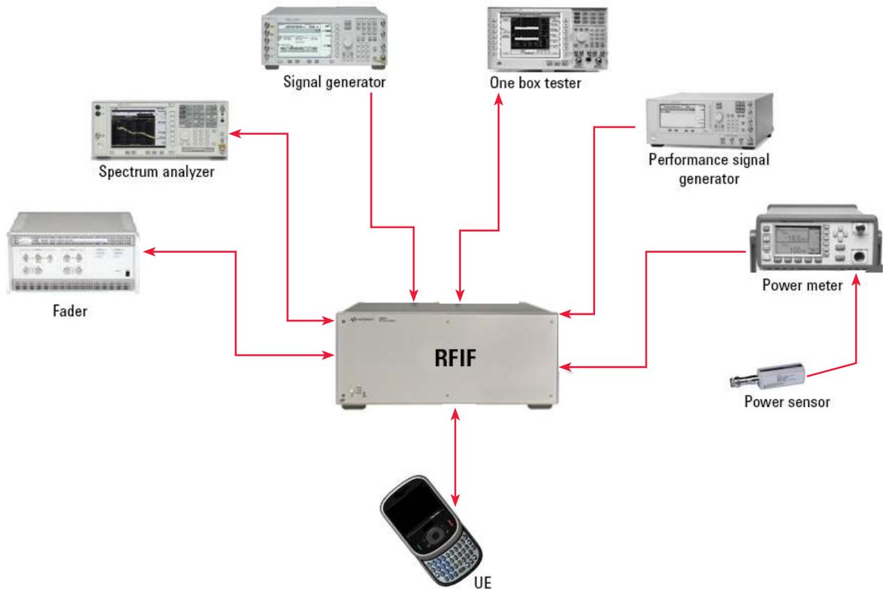
Figure 1. Components of the GS-8800 conformance test system
