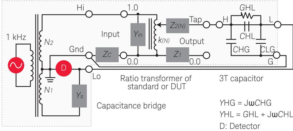
Figure 3. Equivalent circuit for calibration system.
