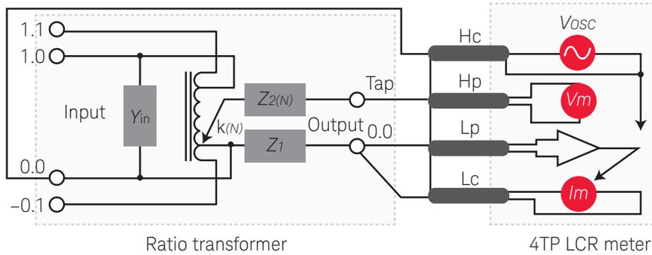
Figure 1. Equivalent circuit for measurement of  $Z_1$ .
