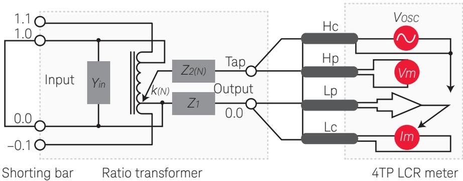
Figure 2. Equivalent circuit for measurement of  $Z_{2(N)}$ .
