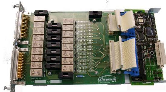
Figure 2. Keysight 34959A breadboard module with LXinstruments circuitry.
