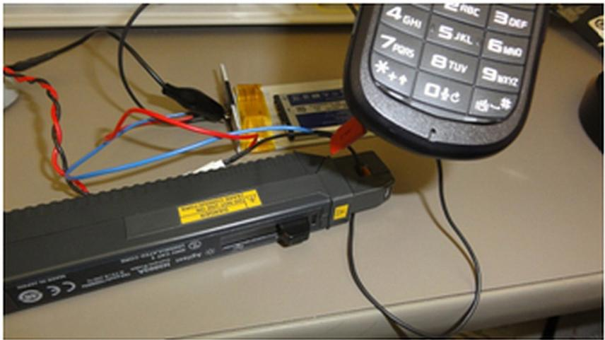
*Figure 2 A simple way to measure a current with an oscilloscope is to use a clamp-on type current probe such as Keysight's 1147B or N2893A.*
