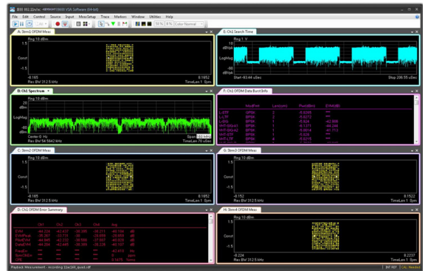
Figure 3. Results on M9703A of BBIQ MIMO analysis with 89600 VSA software.
