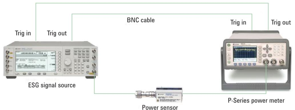
Figure 2. Two-way communication external triggering setup diagram
