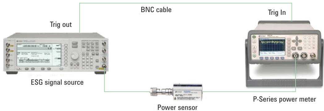
Figure 1. One-way communication external triggering setup diagram
