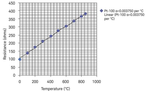
Figure 6. Linear (pt-100  $\alpha = 0.00385$  per  $^{\circ}\text{C}$ )
