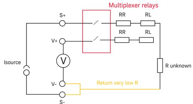
Figure 5. Three-wire technique.
