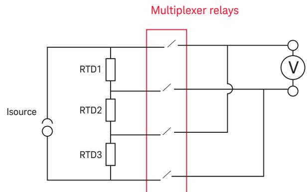
Figure 7. Series RTD configuration with external current source.
