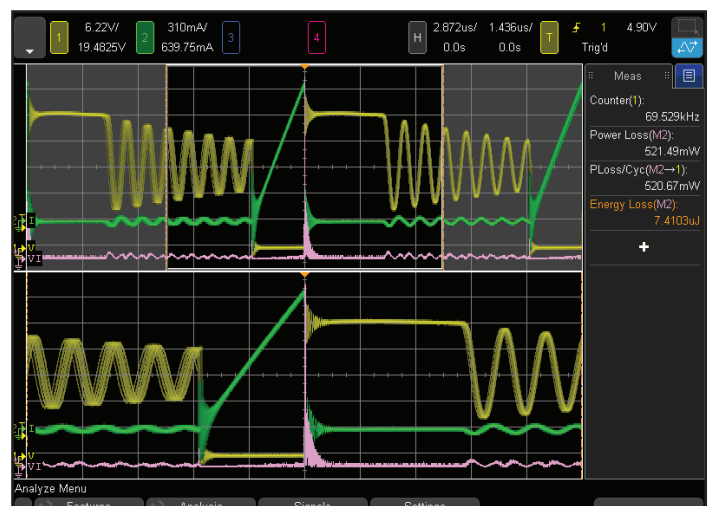
Figure 3. Automatic power and energy switching loss measurement performed by a Keysight oscilloscope.
