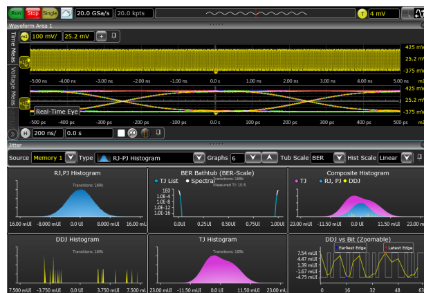
Figure 12. Real-world jitter measurements using Infiniium S-Series oscilloscopes. All models in the family utilize the same time base technology block and a low horizontal component of jitter measuring less than 130 fs over short record lengths.
