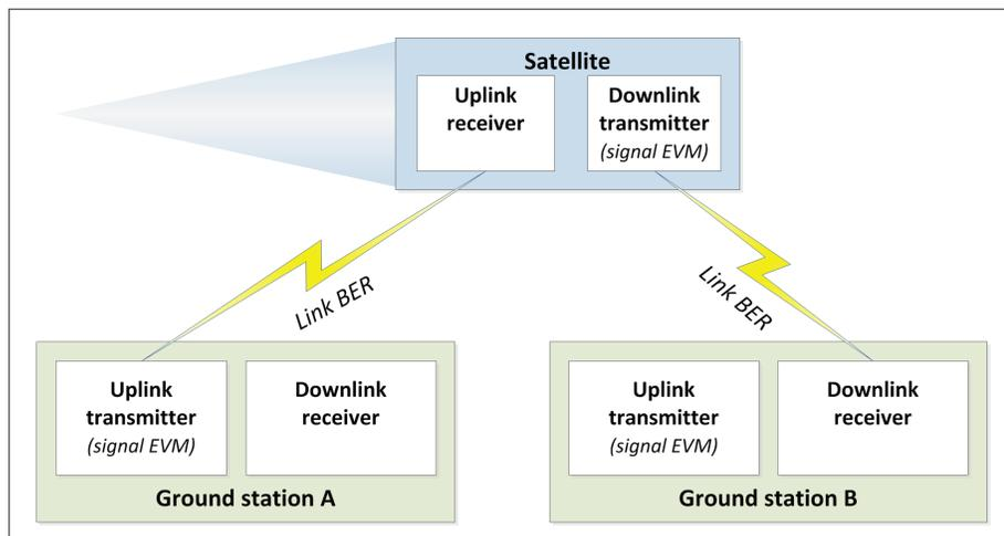
Figure 1. Link BER defines the end-user's experience while EVM characterizes the signal quality of analog and digital modulated signals.
