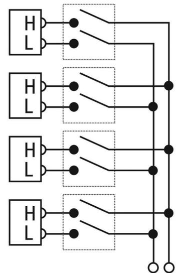
Figure 3. Shown here is a 2-wire, 4:1 MUX.
