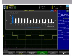
In addition to the harmonics table, simultaneously view a bar graph of the harmonic orders to visually identify high-value harmonics.
