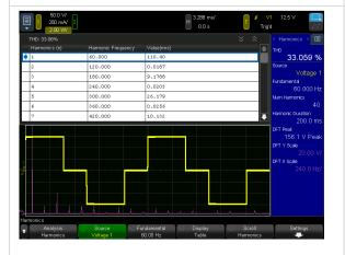
Figure 9. Harmonic measurements with graph
