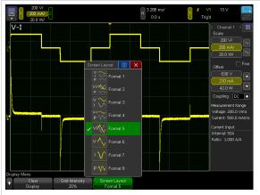
Figure 10. User selectable screen layouts
