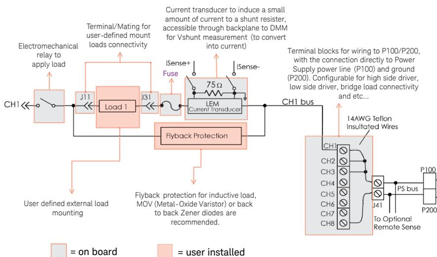
Figure 5. E6178B load switching channel 1
