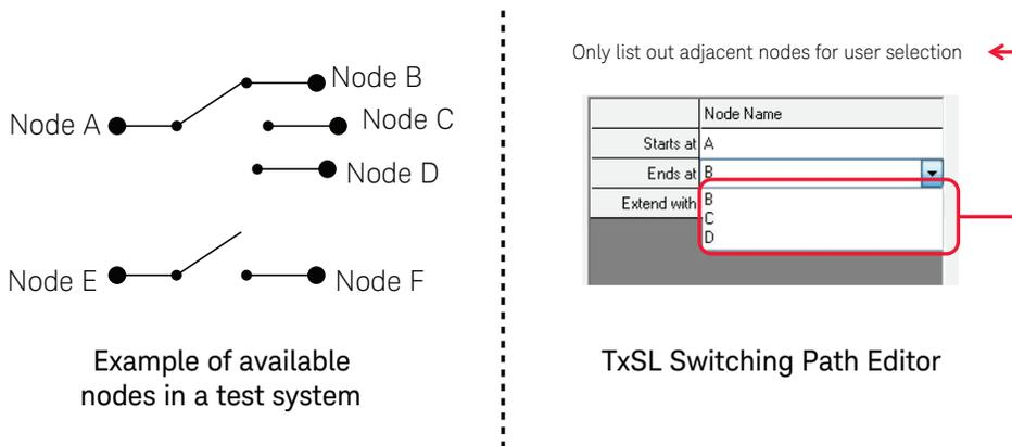
Figure 3. An example of using TxSL Switching-Path-Editor
