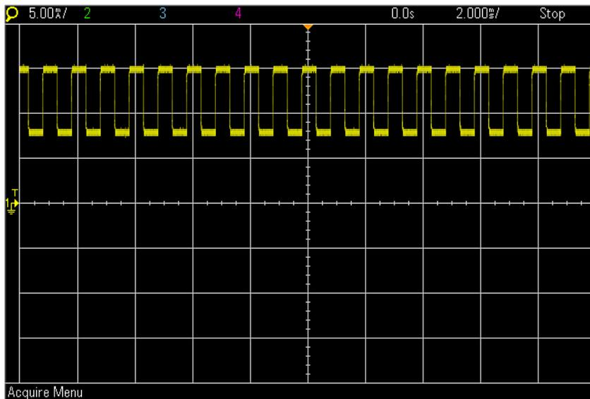
Figure 4. 1 kHz current pulse signal generated by a wheel speed sensor
