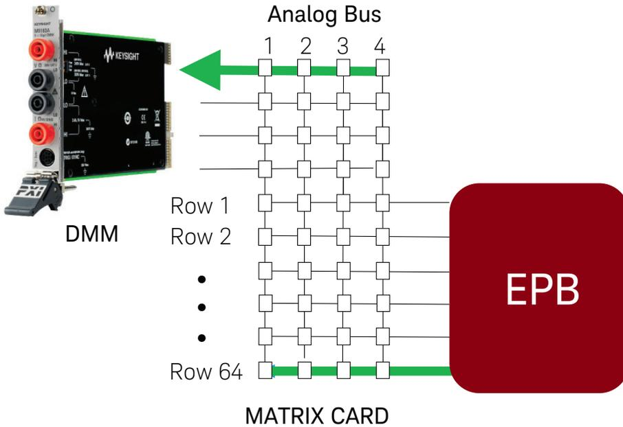
Figure 2. Pin matrix card connection for DMM accessibility
