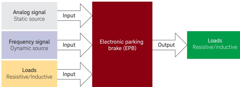
Figure 1b. Respective models for functional testing of EPB functionality
