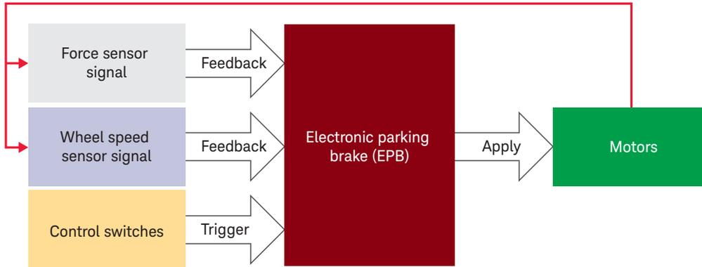
Figure 1a. Simplified block diagram of EPB operation
