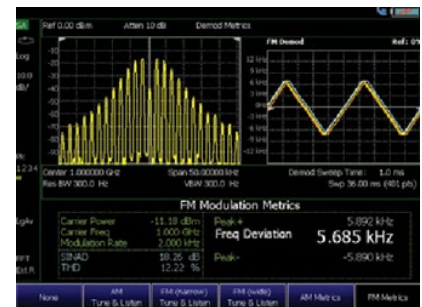
Characterize AM/FM signals using AM/FM demodulation
