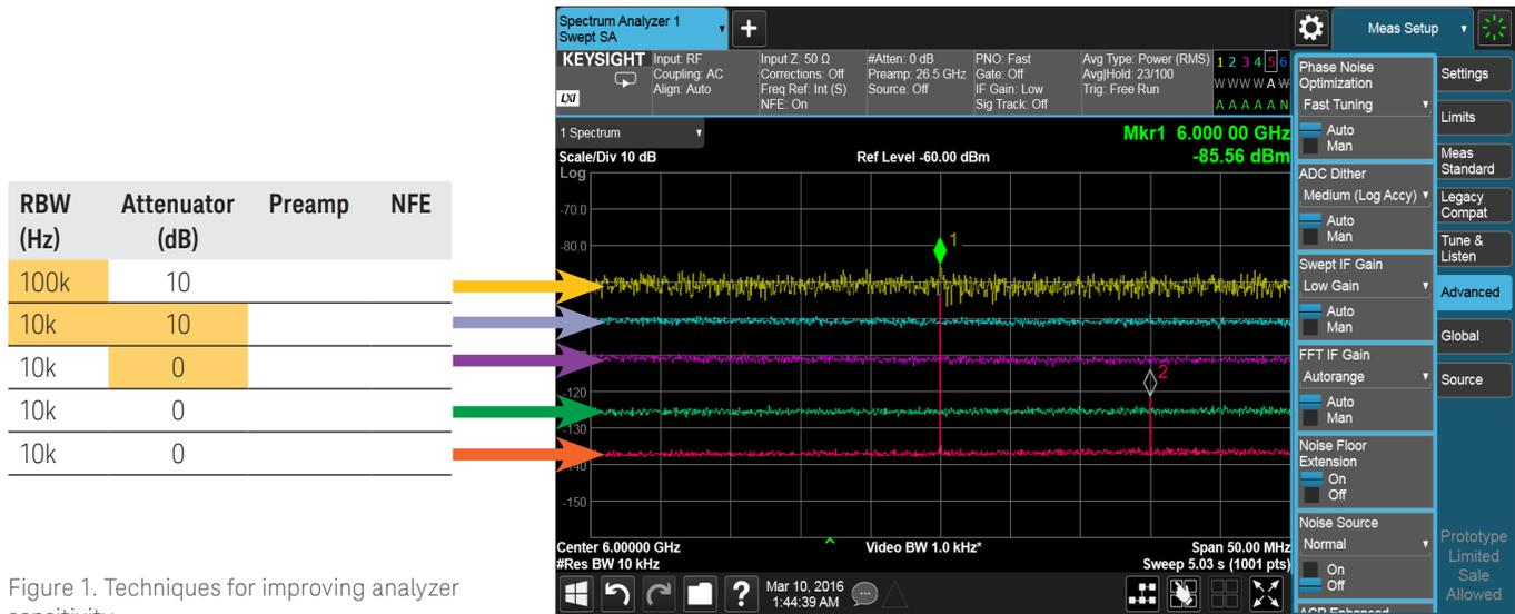
Figure 1. Techniques for improving analyzer sensitivity.
