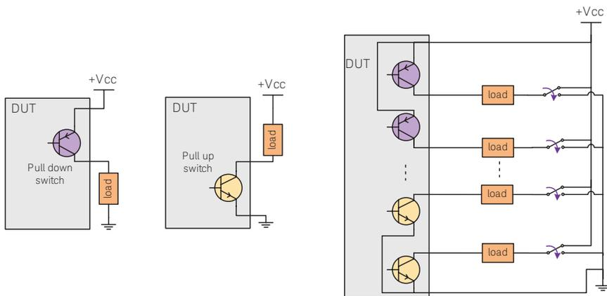
Figure 6. High side driver and low side driver and its equivalent switching for power or ground in a complete circuitry
