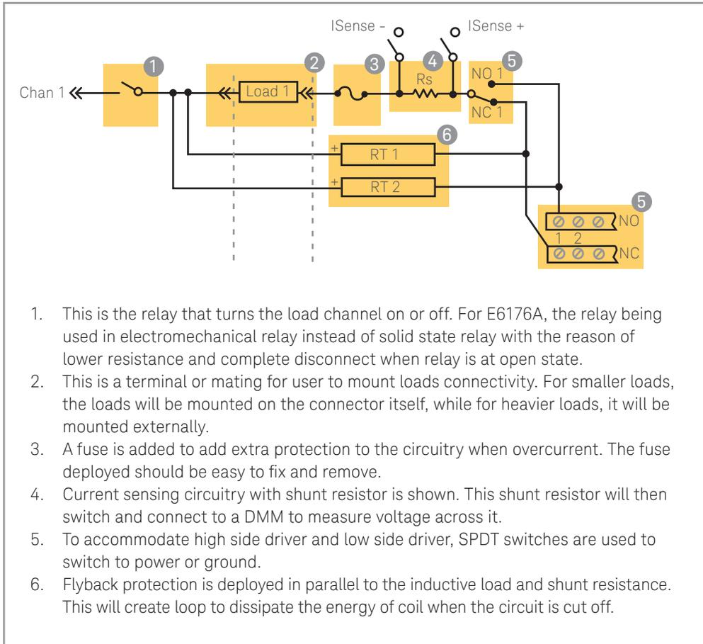
1. This is the relay that turns the load channel on or off. For E6176A, the relay being used in electromechanical relay instead of solid state relay with the reason of lower resistance and complete disconnect when relay is at open state.
