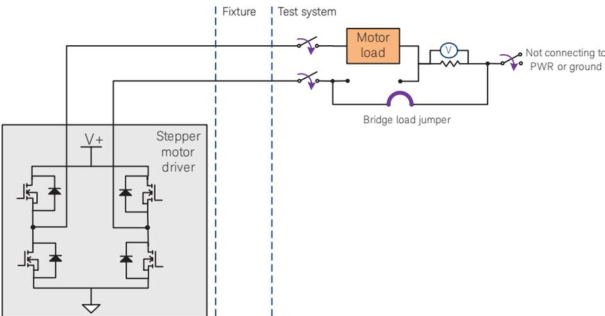
Figure 8. Bridge load for stepper motor application
