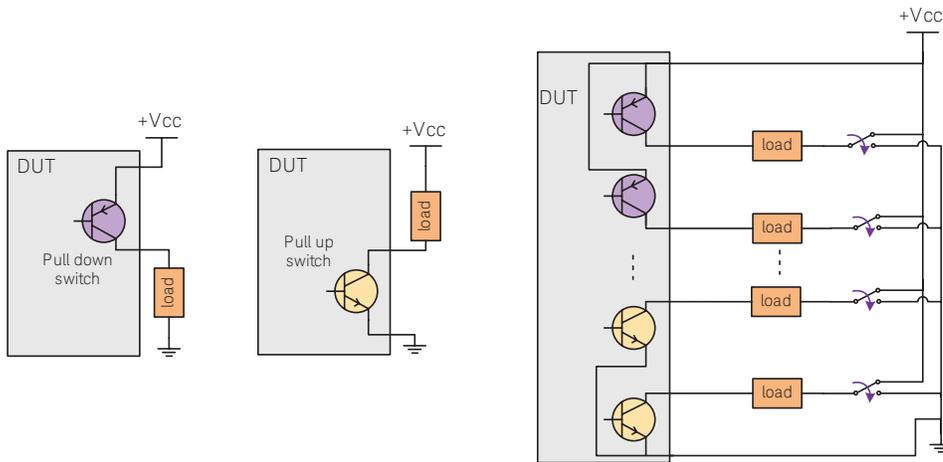
Figure 7. Multiple load configuration for load channels which is suitable for output leakage test
