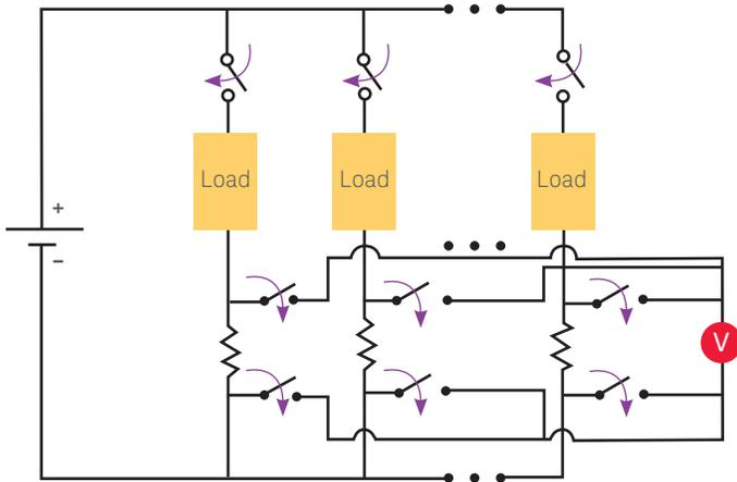
Figure 4. Shunt resistor method of current measurement
