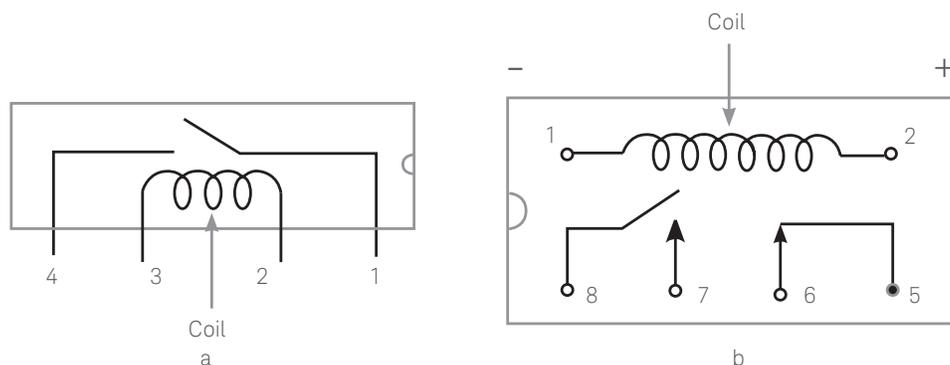
Figure 1. Electromechanical Relay (a) single pole single throw, (b) single pole double throw
