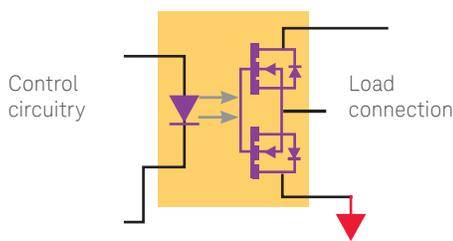
Figure 2. Solid state relay
