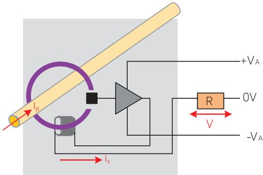
Figure 5. Close loop current transducer (extracted from LEM website)
