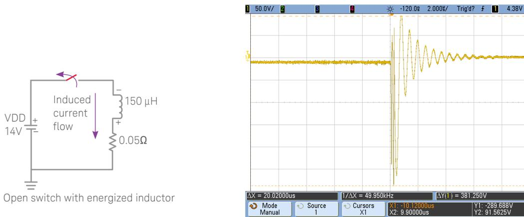
Figure 9a. Flyback is observed on digitizer when switch is opened.
