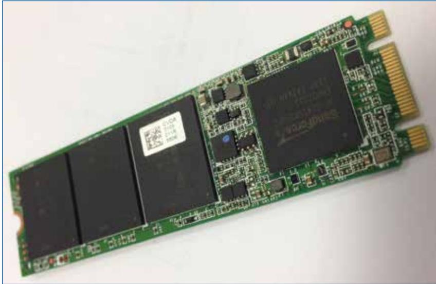
FIGURE 1. M.2 SSD for tablet and laptop PC, the smallest commercial version.
